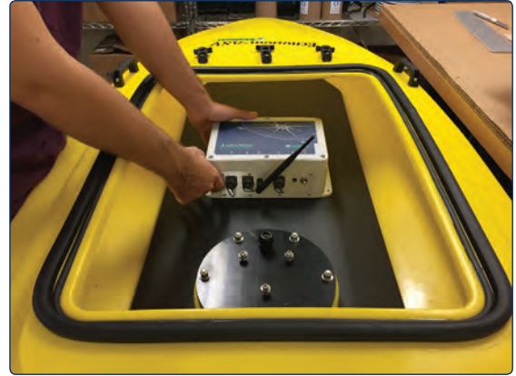
Transducer well and AutoNav™ shown in the EchoBoat hull
