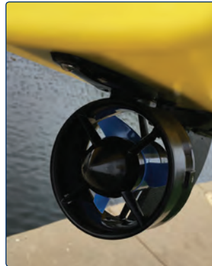
Powerful differential thrusters for maneuverability
